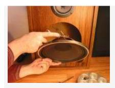
Check to make sure the wires from the terminal block at the rear of the speaker enclosure are connected to the back of the driver.
