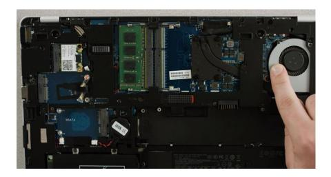
Turn off the computer, unplug it, and remove the battery by moving the locking slider to the unlock position. There will be another slider, move it in the direction indicated, then pull the battery straight out. Press the power button for at least five seconds to discharge any remaining electricity in the system.
