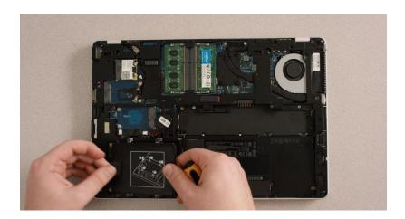
Remove the memory modules by pressing down on the clips that hold each module in place, using your fingers or a spudger tool. The module will pop up at a 30-degree angle, allowing you to remove it. Don't touch the gold pins on the module.
